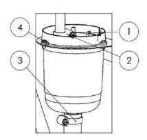
Fig. 6-4. Humidifier water level detector
