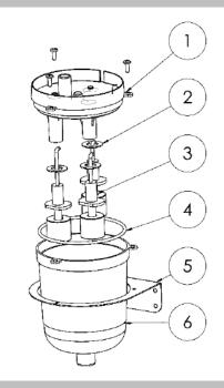
Fig. 7-3. Water level detector exploded view
