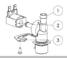
Fig. 7-2. Water inlet valve exploded view
