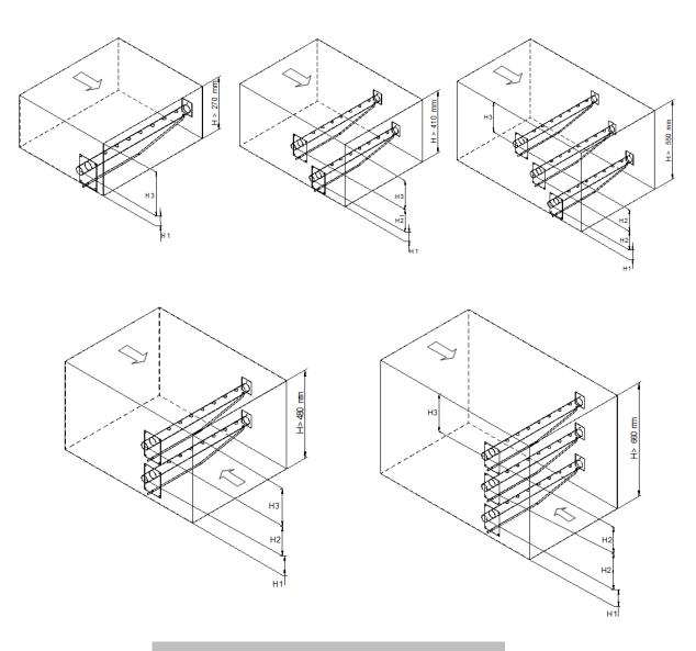
Fig. E 3-3. Minimum heights & flow directions
