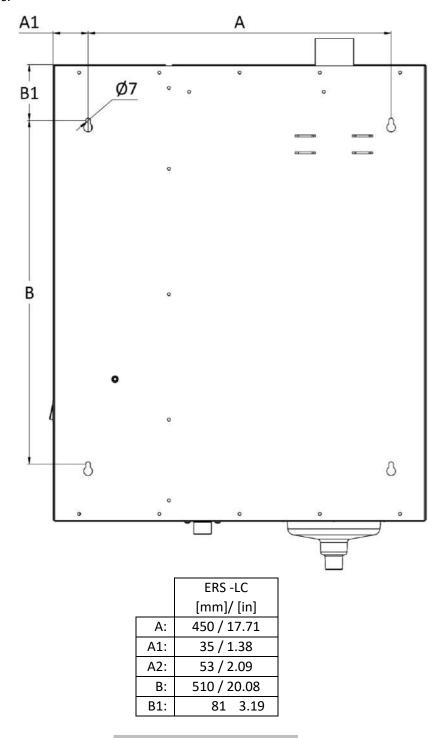
Fig. 3-1. Installation holes
