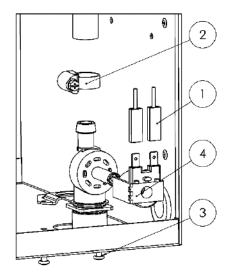
Fig. 6-3. Humidifier water inlet valve
