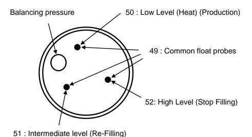
Fig. D 3-8. (OPTION) ELECTRODES LEVEL DETECTOR
