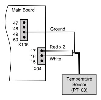
**2. Defective temperature sensor.** Disconnect the temperature sensor from connector X04. Use a multimeter to measure the resistance value of the PT100 at room temperature and compare this value with the PT100 resistance table.
