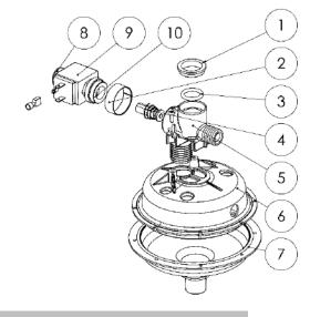
Fig. 7-4. Draining circuit exploded view
