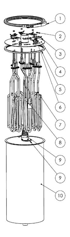
Fig. 7-1. Tank exploded view
