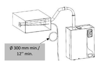
Fig. A 3-4. Standard installation
