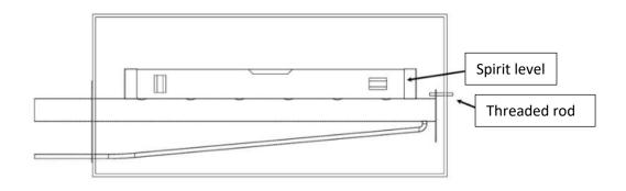
Fig. A 3-3. Steam dispersion tubes positioning
