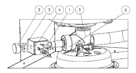
Fig. 6-2. Humidifier drain valve
