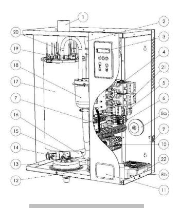
Fig. 2-3. Humidifier component parts
