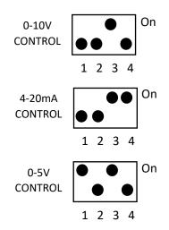
Control signal type setting in humidifier menu
