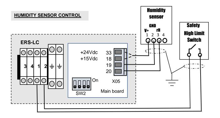
SW2 Dip switch setting to do on main board
