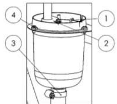
Fig. 6-4. Humidifier water level detector
